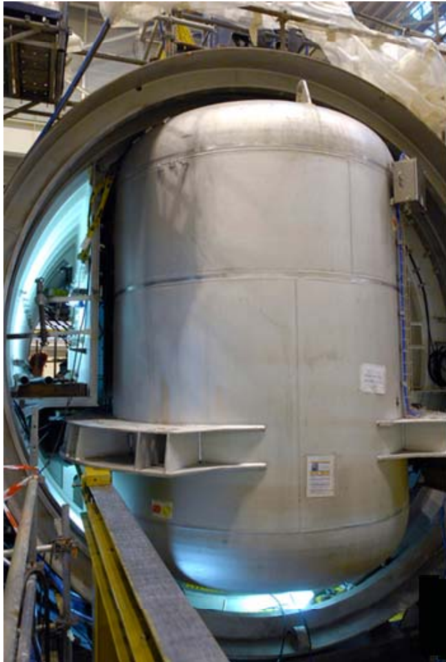
AIP "MESMA" with Vertical and Horizontal options of LOX Tank. French SSK submarines SCORPENE and AGOSTA-90B are fitted with AIP "MESMA"
